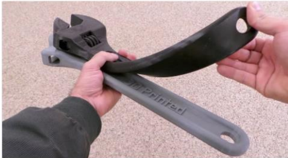
When you want to print with flexible materials, direct drive is recommended (Source: Creative Tools via YouTube )
